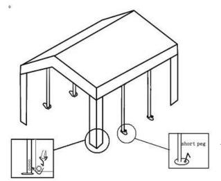
IV Attach the another 4 supported poles (3) to the joints (4,5), built-up the framework ,use the 6x180mm peg to fix each
