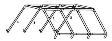
II Attach one end of supported pole (3) to the joints (4,5)
