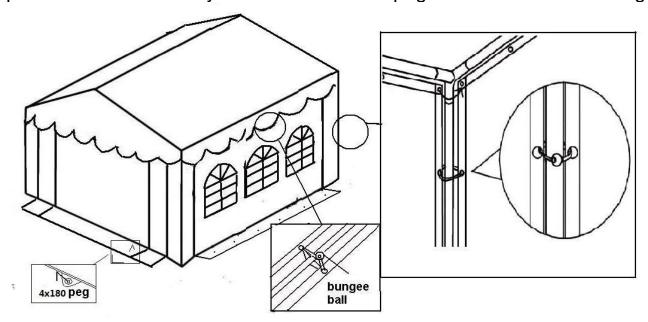
**VI** The Guy lines clasp to each corner of tent and another end of line fix to ground by pegs 8x300mm
